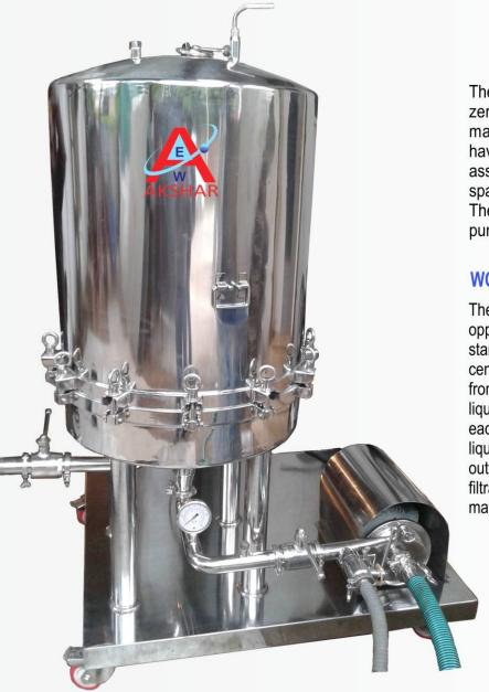
The **AKSHAR** manufacturer and supplier of zero hold up filter press in India that is made up of high quality stainless steel having customized finished design. The cartridge assembly consists of plates, perforated screens, spacers and fitter media stands on S.S. trolley. The whole assembly complete with attached pump and pipe lines through welding.
