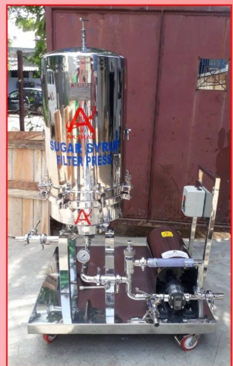
Sugar Syrup Sparkler Filters 14" x 15 Plates Rotary Gear Pump
