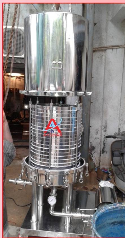
Sugar Syrup Sparkler Filters 14" x 15 Plates Rotary Gear Pump
