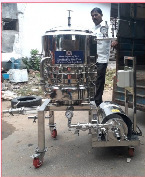
Jacketed Sparkler Filters 14" x 8 Plates Centrifugal Pump
